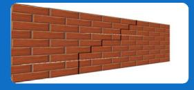
Push the helical bar firmly into the grout, making sure that the bar extends 500mm either side of the crack.
